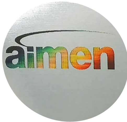
Figure 5. Picture of an AIMEN's logo engraved on the surface of a stainless steel sample by using a 6 \mu\text{m} period laser interference pattern.
