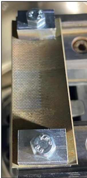
Figure 5: DLW textured cylinder liner segment and 3D and sectional profiles of Texture 2
